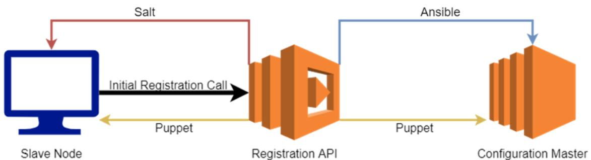
Fig. 4.2 **Registration API behaviour by tool**
